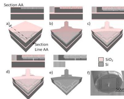
Figure 2 Probe fabrication. a) Patterning of the measurement mirror. b) Patterning of the supporting tabs. c) Release of the measurement mirror. d) Patterning of the reference mirror. e) Release of device. f) Scanning Electron Microscope (SEM) image of the final device.
